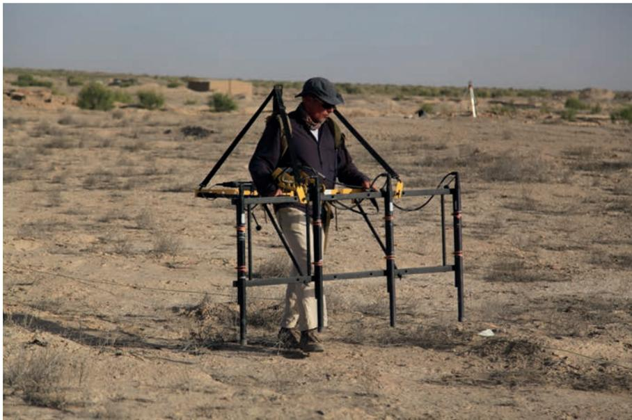
Fig. 1: Fluxgate-Magnetometer mounted on a portable rack, Gonur Depe (photo C. Hübner).
