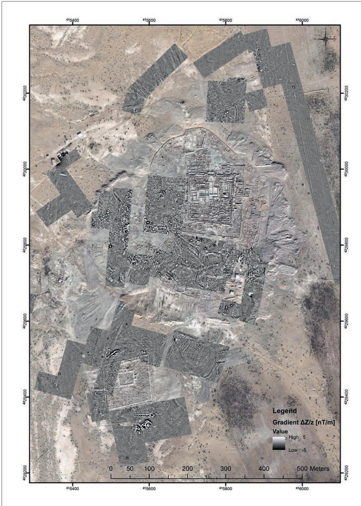
Fig. 2: Magnetogram of Gonur Depe North and the *temenos*; area 257,712 sq m; Förster gradiometer; measuring grid: 0.5 x 0.2 m; dynamic range [ $\pm 5$  nT] combined with World Imagery, Sources: ESRI, DigitalGlobe, GeoEye, i-cubed, USDA FSA, USGS, AEX, Getmapping, Aerogrid, IGN, IGP, swisstopo, and the GIS User Community.
