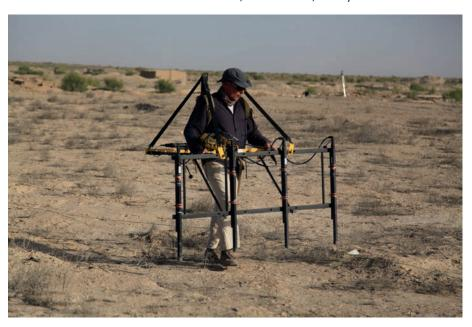
Fig. 1: Fluxgate-Magnetometer mounted on a portable rack, Gonur Depe (photo C. Hübner).
